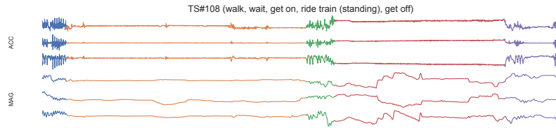
Fig. 1. MTS from the HAS challenge benchmark [4]. The different channels show sensor signals capturing a student commuting to university, with activities colour-coded. Only a subset of dimensions is relevant for HAS.
