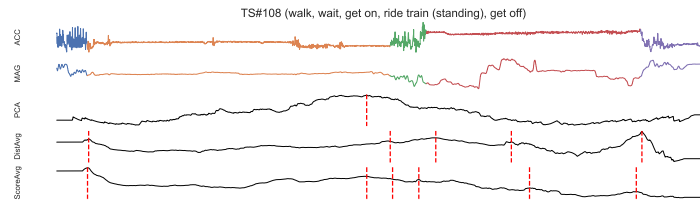
Fig. 8. Top-2: X-axis acceleration and magnetometer from Figure 1 (activities are differently coloured). Bottom-3: ClaSP profiles created using PCA, distance and profile averaging. CPs are illustrated as red bars. Distance averaging shows best results.
