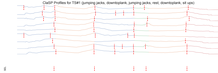
Fig. 6. ClaSP profiles for the TS from Figure 3 (light colours). All found CPs are illustrated as red bars. Single channels contain false or missing predictions. The bottom CPs are the filtered selection and correctly capture the activity transitions.
